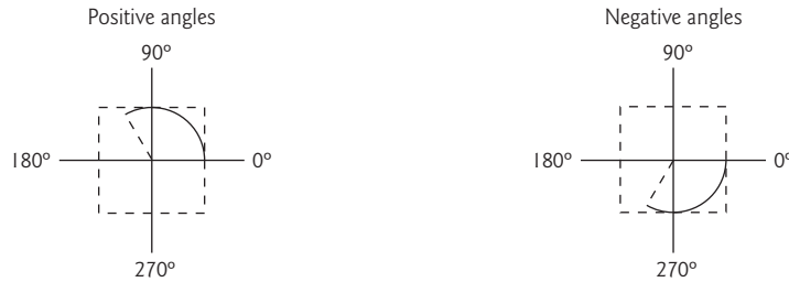
Fig. 27.22 | Positive and negative arc angles.
