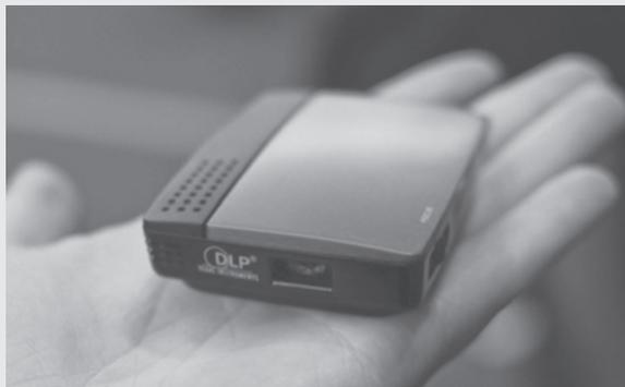
**FIGURE 29.9** A prototype pico projector based on DPT.
